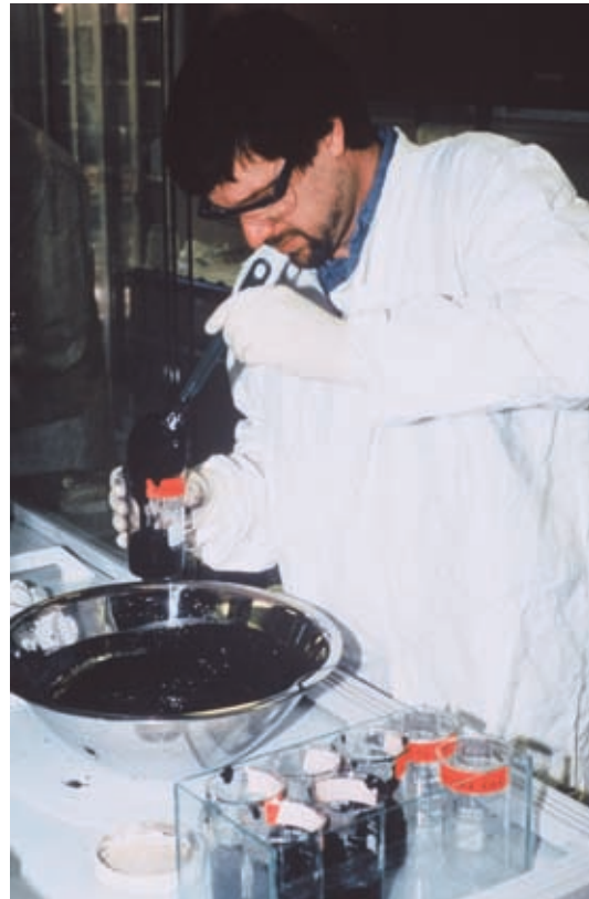
Subsampling sediment for toxicity testing
