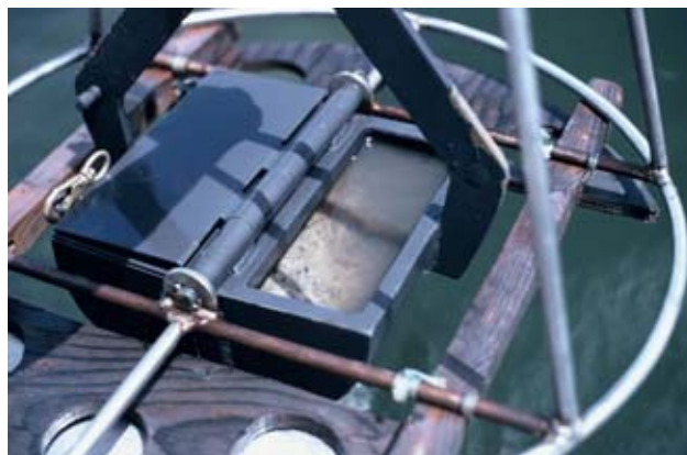
Ted-Young VanVeen sampler in supporting frame. Illustrating movable cover flap to enable direct sampling from the grab sampler. Note the overlying water in the sampler and adequate volume, indicating an acceptable grab sample.
