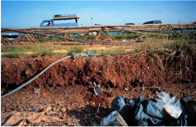
Figure 2. A view of mine-waste calcines that were used to construct the jetty in Honda Bay. This photo is at the waterline in Honda Bay and in the background are fish drying racks and motor vehicles.
